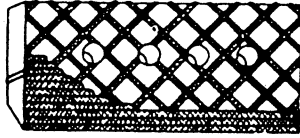
Figure 7-48.—Wearfacing bulldozer end bits.
